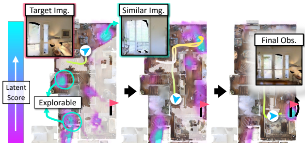
Figure 5. Example of image-goal navigation episode. The heatmap value of E from F_{loc} is highlighted on the map according to the colorbar on the left.
